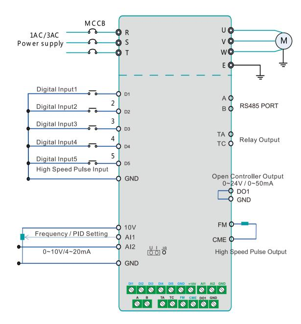
Digital Input X 5 [D1 ~ D5] Relay Out put X 1 [TA,TC] HDI (High Speed Pulse Input /Output ) X 1 [D5/FM.CME ]
